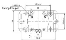
A, a - Main/Direct connection port, jaw opening B, b - Main/Direct connection port, jaw closing
